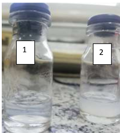
Fig. 1: Aluminum hydroxide gel sample with 1.5% trehalose after treatment with ultrasonication for 30 min with setting intensity 3 in the presence of ice the sample becomes clearer by time and the viscosity changes (1), control sample without treatment (2).
